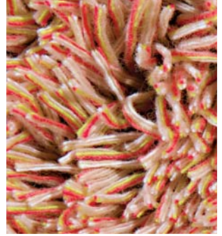
Quintet yarn with four different colors in a shag pile.
