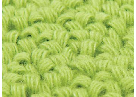
Sextet yarn in a high loop pile with six ends of lime green.
